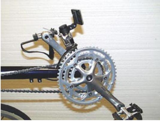
After cutting the chain to the correct length, re-route the chain through the rear derailleur. Move the chain and derailleurs to the smallest chainring in the front and the smallest cog in the rear to allow for easier reconnection. After verifying that the chain is routed through the derailleurs, idlers and pulleys correctly, reconnect the two ends of the chain.
