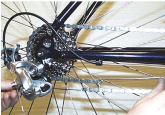
Next, break the chain using the quick link or your chain tool and unwind the chain from the rear derailleur pulleys. (Note: Chain must still be routed through the frame idlers.) With the chain on the largest sprockets, pull the two ends of the chain together. Add or remove enough chain links to achieve at least a ONE (but not more than TWO) LINK OVERLAP (see picture at left)
