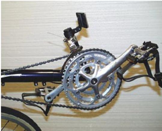
First make sure you have enough chain for the "big / big" combination. (Largest chainring and largest cassette cog). The following must be done with your bike on a repair stand or a friend holding the bike so the rear wheel is off the ground. **Do not attempt to do this while riding because, if there is not enough chain, you will damage your bike.**
