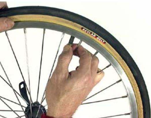
**Step 11:** Pull the valve stem back out, and make sure it is straight. If you have a threaded presta valve, you might want to affix the valve nut to hold the valve steady.
