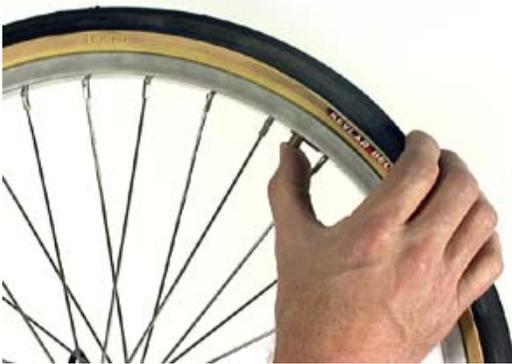
**Step 10:** Before inflating the tire, push the valve stem into the tire to ensure the valve base is inside the bead. If you don't the innertube will lift the tire off the rim as you inflate it.
