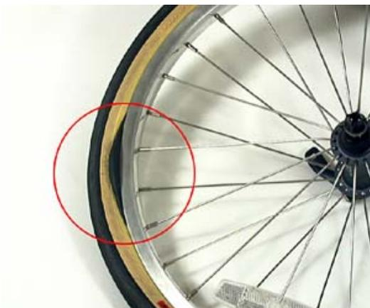
**Warning:** This picture shows the innertube beginning to bulge out from under the tire after inflation. About 5 seconds from this point, the innertube will expand quickly out, lifting the tire off the rim before blowing. Most high pressure tires have enough pressure to blow the sidewall out of a brand new tire, so inflate your tires slowly to their *recommended* pressure while looking for areas where the tire is not seated properly on the rim.
