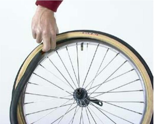
**Step 5:** Working from the valve stem, start tucking the innertube into the tire with your fingers.
