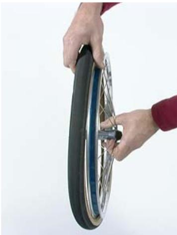
**Step 2:** Starting with the tire alone (no tube), line up the decal on the tire with the valve hole in the rim. Some cyclists like to align the inflation pressure information with the valve stem. Either way, if you always install your tires the same way, it will help you determine the puncture location in the event of a flat tire.
