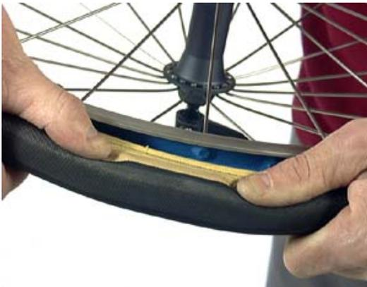
**Step 13:** Now, deflate the tire enough so that you can squeeze the bead away from the rim sidewall, as shown. Starting at the valve, work your way around the tire, squeezing as you go, making sure that the tube is seated in the tire completely. Flip the tire over and repeat.
