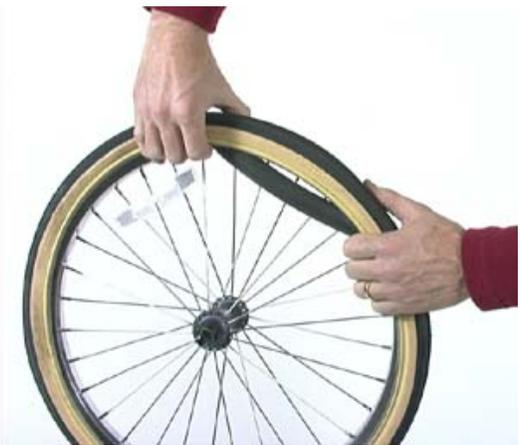
**Step 6:** Work your way around the tire, ensuring that the tube is evenly distributed in the tire. If you have extra tube at the end, or not enough, re-check that you have the correct diameter innertube. Do not fold an innertube over to make it fit!
