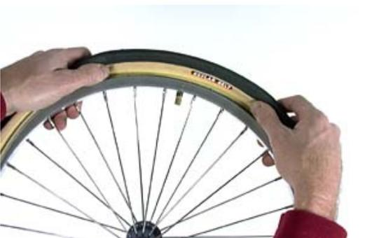
**Step 7:** After your tube is inserted into the tire, start at the valve hole again and begin working the remaining bead onto the rim. Ensuring that the bead is pushed tightly down into the rim as you go will make the final bead "pop" much easier.
