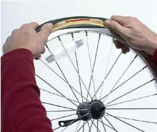
**Step 9:** Many beads will be very tight for the last few inches, but you should avoid using tire levers if at all possible. Being persistent with your thumbs will almost always work. If the last bit of the bead seems impossibly tight, go back to the start of the bead installation and make sure you have the bead as tight as possible all the way up to the final few inches and that there isn't any innertube wedged between the tire bead and rim.
