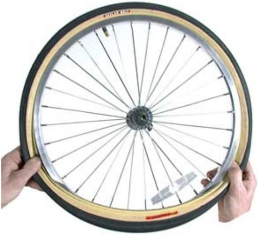
**Step 8:** Using both hands opposite each other, continue working the bead onto the tire, making sure the bead is tight against the rim.
