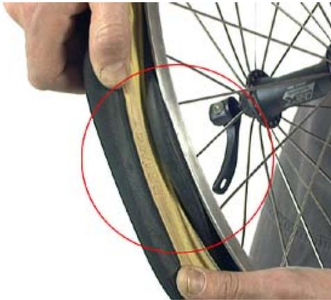
**Warning:** This picture shows a section where the innertube is between the bead and rim. If this occurs, pinch the tube and tire together with your fingers and work them around until the tube works its way back inside. *DO NOT* use a tire lever or other object to "stuff" the tube back in.
